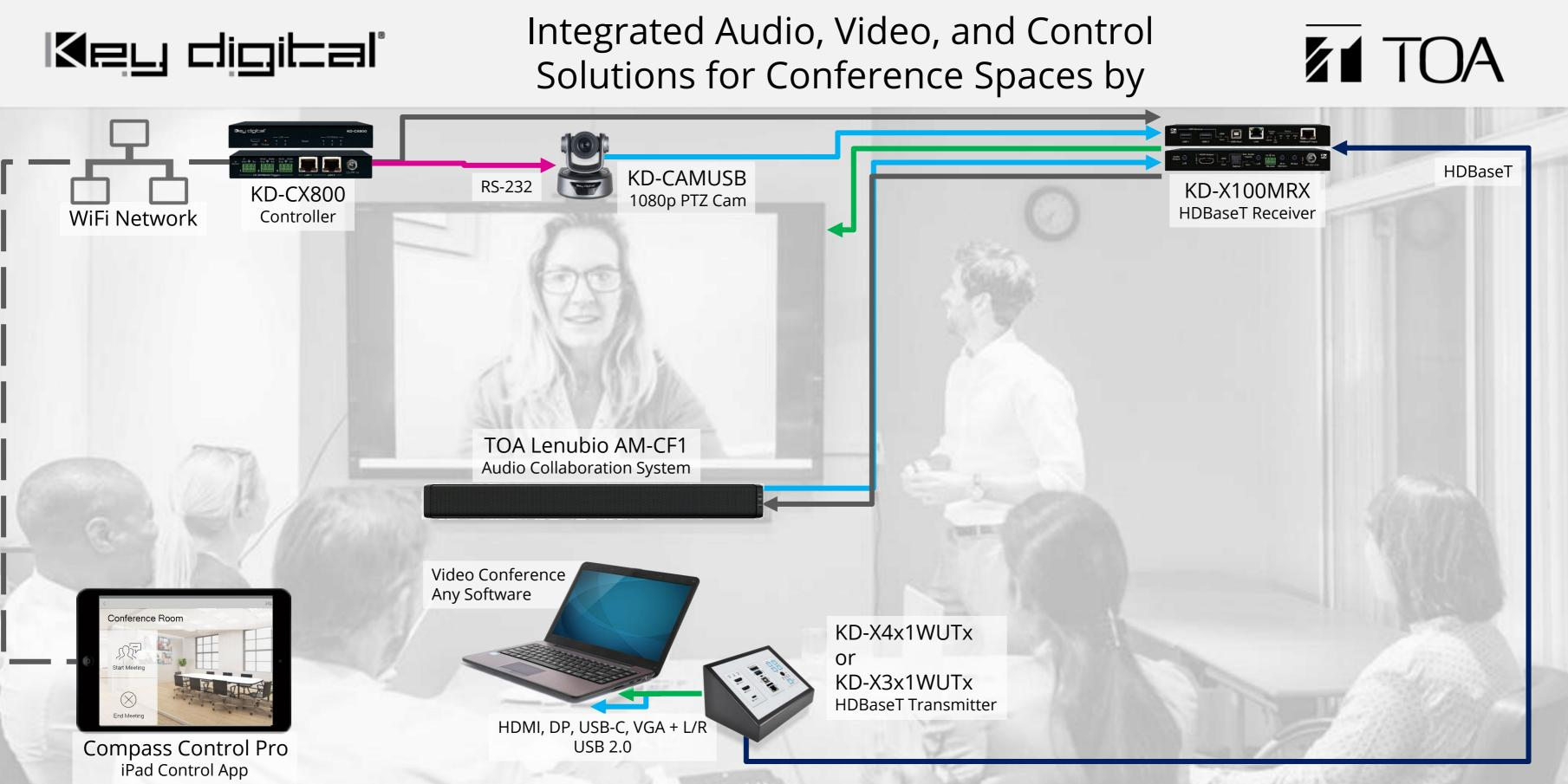
Kit 3 / Best 1: HDBaseT Consolidation & 100m Extension of Audio, Video, USB Products shown: TOA Lenubio, Key Digital KD-X4x1WUTx / KD-X3x1WUTx, KD-X100MRx, KD-CamUSB, KD-CX800, KD-ProCL1 System Delivery: Connect laptop USB and AV to present and provide remote participants an HD 1080p professional auto-PTZ controlled view of the conference space while speaking with each other just as they would in normal conversation thanks to the integrated array mic and soundbar.
