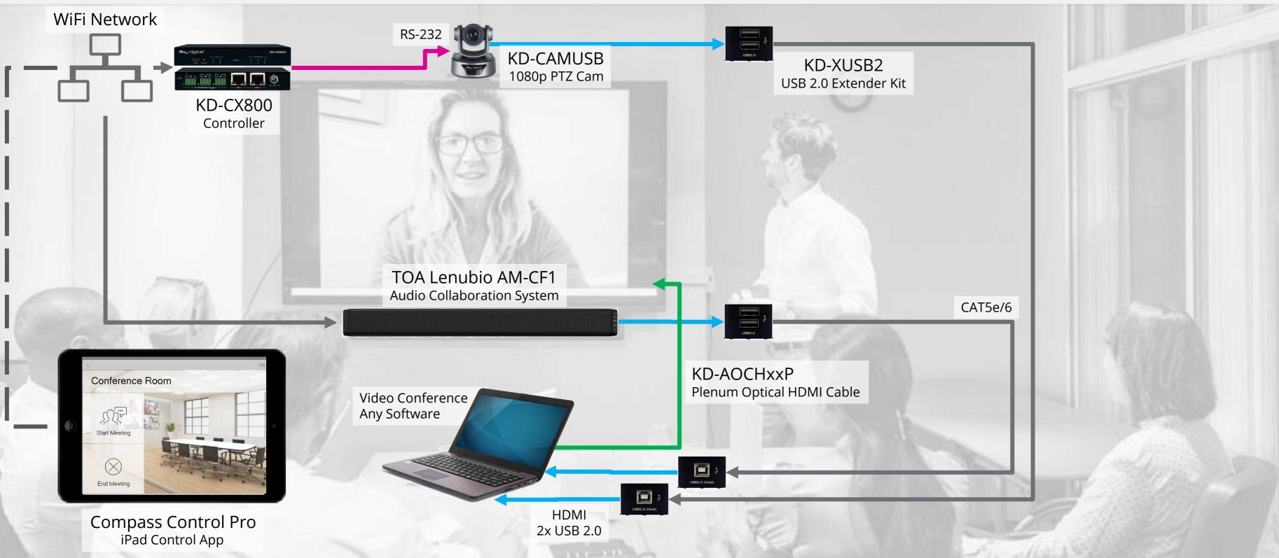
**Kit 2 / Better:** ≤ 50m / 164ft USB & HDMI cable length from Display Products shown: TOA Lenubio, Key Digital KD-CamUSB, KD-CX800, KD-XUSB2, KD-AOCHxxP, KD-ProCL1 System Delivery: Connect laptop USB & HDMI to present and provide remote participants an HD 1080p professional auto-PTZ controlled view of the conference space while speaking with each other just as they would in normal conversation thanks to the integrated array mic and soundbar.
