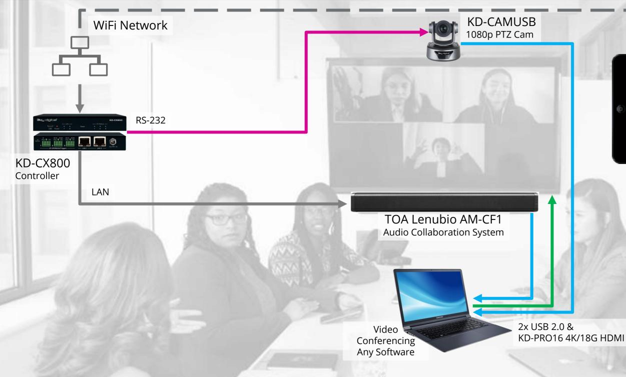
**Kit 1 / Good:** ≤ 5m / 16ft USB & HDMI cable length from Display Products shown: TOA Lenubio, Key Digital KD-CamUSB, KD-CX800, KD-Pro16, KD-ProCL1 System Delivery: Connect laptop USB & HDMI to present and provide remote participants an HD 1080p professional auto-PTZ controlled view of the conference space while speaking with each other just as you would in normal conversation thanks to the integrated array mic and soundbar.
