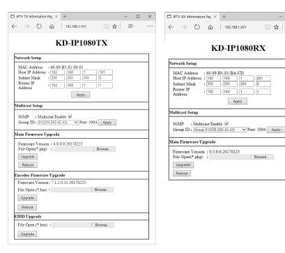
Once connected, the KD-IP1080 web interface would look like this (Tx on left, Rx on Right). Network Setup, Multicast Setup, and Main Firmware Upgrade are the same for both Tx and Rx units.
